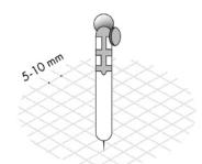
The test gives information regarding the resistance of the surface of the base screed, which is fundamental in order to avoid working on a surface which isn't compliant with the minimum performance levels required. It is a simple test that requires minimal experience and manuality and presents results which are easy to interpret.
